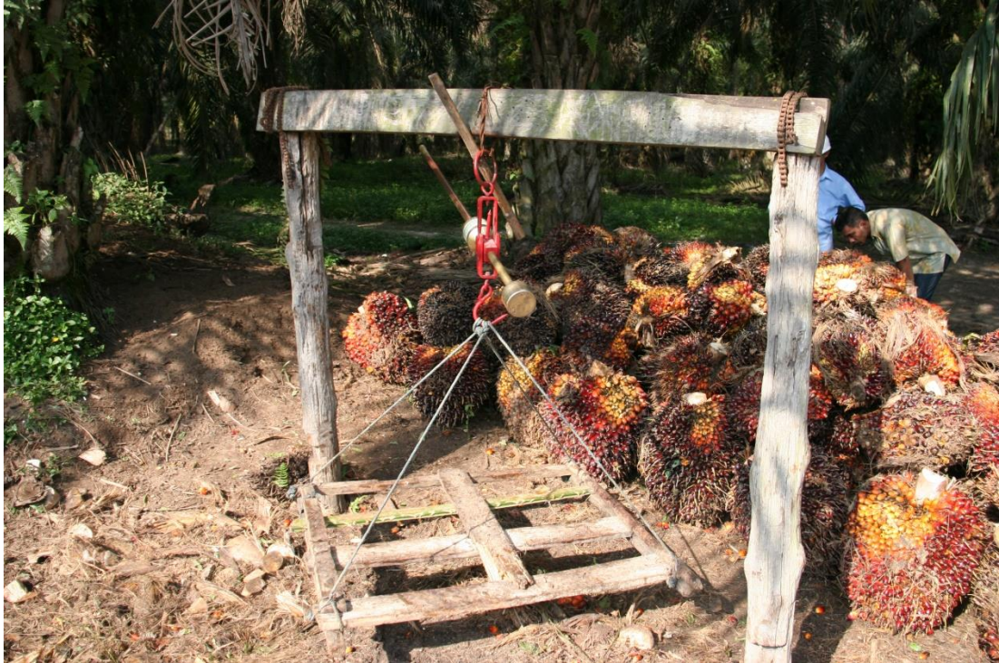
Figure 8: Hanging scales for weighing the bunches. If available, strong digital scales are more precise!
