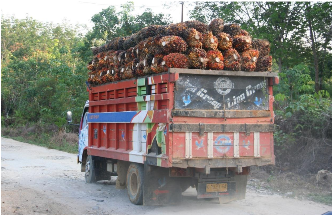
Figure 10: Neatly loaded truck, but the load is too high and should have been covered with a net!
